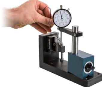
**4.** Set height adjustment screw until dial gauge is set to zero point.
