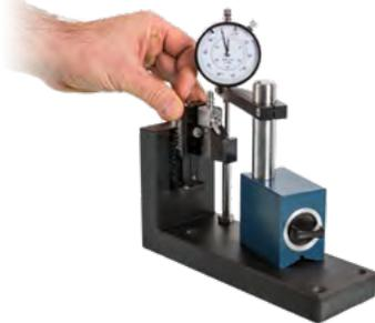
**2.** Place top holder on device and tighten clamping screw slightly until holder sits on device with no play. Ideally, set tip height slightly below centre so that top holder is pulled upwards when height is adjusted.
