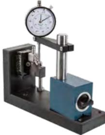
**3.** Carefully place dial gauge on tip of cutting edge.
